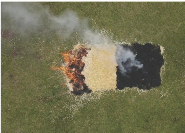
FSI containment line test - simulated straw fire with one section treated with a FSI-Defended product
